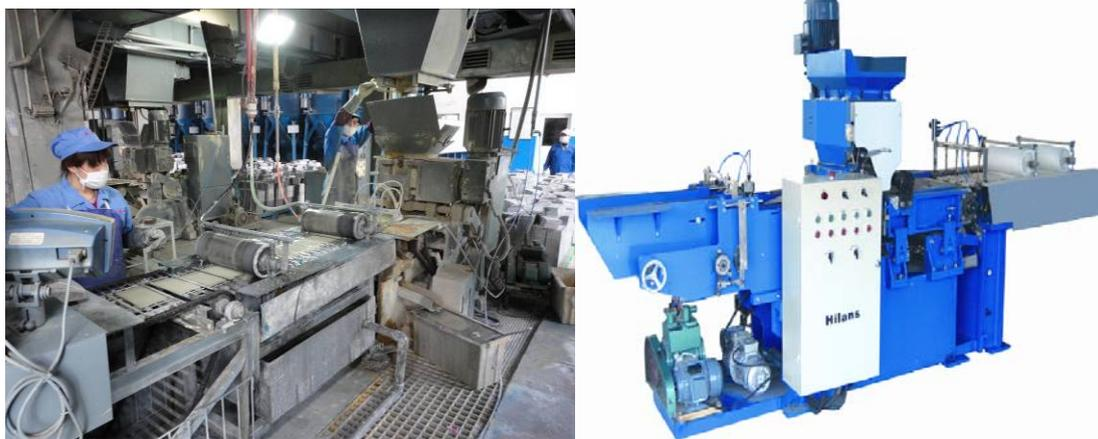
图 6 涂板工序及涂板机
